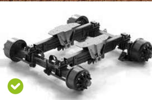
✓ Pendelaggregat Boogie SB
